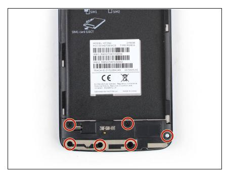
Remove the six 3.3 mm long Phillips #00 screws.
