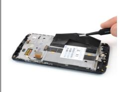
• Use a pair of tweezers to gently peel the adhesive tape off the antenna and interconnect cable and fold it out of the way.
