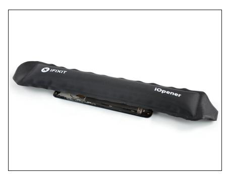
Apply the iOpener for about two minutes on the black adhesive tape that covers the antenna and the interconnect cable.
