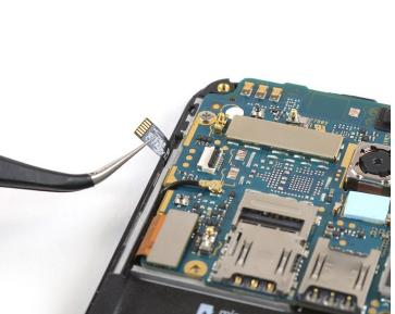
• Slide the volume button flex cable out of the ZIF connector to disconnect it.
