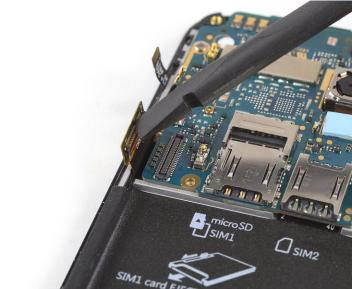
• Use the edge of a spudger to pry up and disconnect the display flex cable located on the bottom left of the motherboard.
