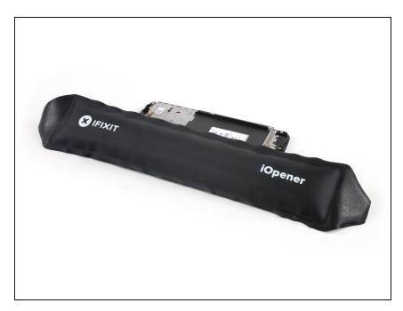
Apply a <u>heated iOpener</u> to the left edge of the phone for about 30 seconds to loosen the adhesive beneath power and volume button unit.
