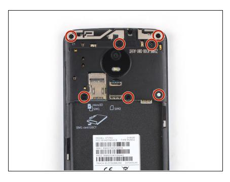
Remove the seven 3.3 mm Phillips #00 screws.
