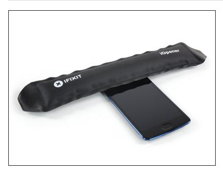
Apply a <u>heated iOpener</u> for about one minute to the upper part of the display to loosen the adhesive beneath the earpiece speaker.
