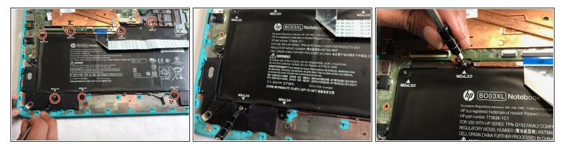
• Remove the seven M2xL3.0 screws from around the battery using a Phillips #00 screwdriver.
