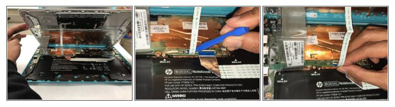
A Lifting the keyboard cover too much may damage the internal cables of the laptop.
