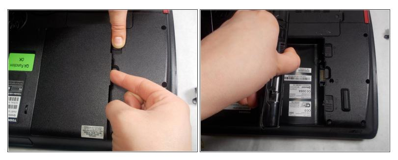
Push tab two in the opposite direction and hold it, while simultaneously lifting battery out of compartment.
