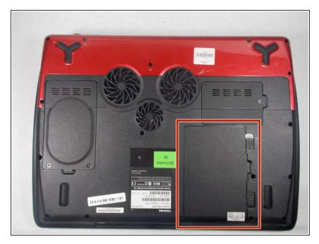
• Flip computer over to expose battery compartment.
