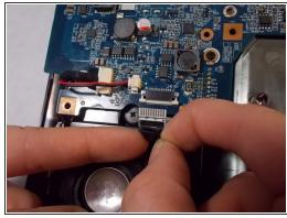
Disconnect all wires from the circuit board.
