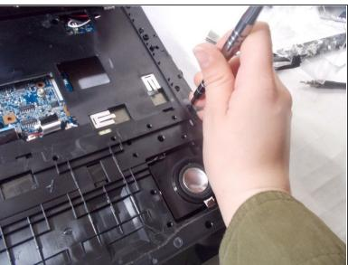
Unscrew the four 10 mm screws with the Phillips #0 screwdriver.
