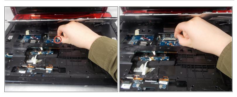
Lift the keyboard up and detach the strip connecting the keyboard to the back of the laptop.
