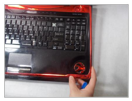
Find an edge of the red strip along the edge the computer and pry it off using a spudger.
