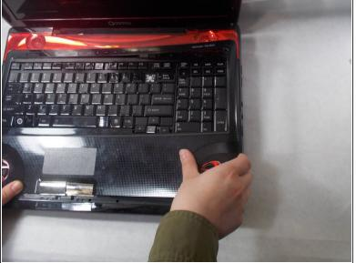
Find an edge of the black cover piece around the keyboard and pry it up using the spudger.
