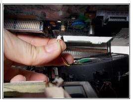
• Disconnect the wire underneath connecting the fan to the circuit board.
