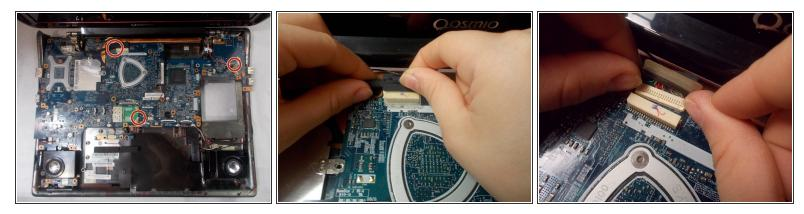
Disconnect all wires connecting the screen to the inside of the computer.
