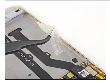
Before installing the new battery, be sure to remove any broken adhesive strips that were left behind.
