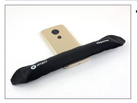
• Use the iOpener to heat the back of the phone along its bottom edge for about two minutes, or until it's slightly too hot to touch.
