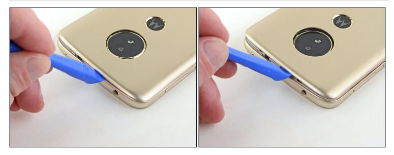
• There are some areas around the edge that are held down with plastic clips. The opening pick should detach most of the clips. If not, insert an opening tool into the gap and pry the back cover up to release the clips.
