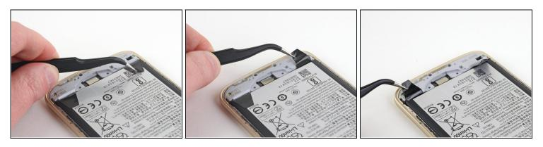
• Use a pair of tweezers to peel up the two battery adhesive tabs at the bottom of the battery.
