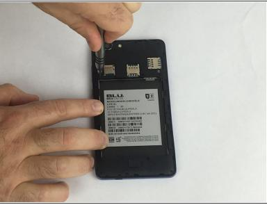
Remove the 12x3mm screws from the rear plate using the Phillips#000 screwdriver.
