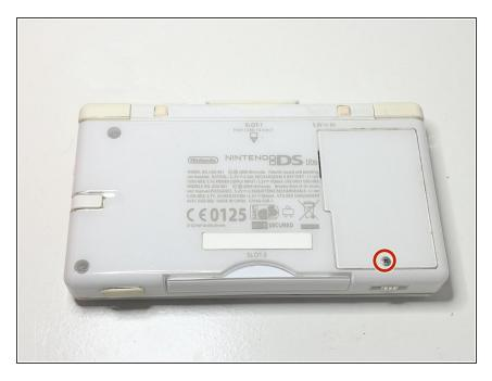
Use a Phillips #00 screwdriver to remove the screw securing the battery cover.
