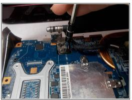
Remove the 6 mm screws holding the screen on to the laptop using a Phillips #0 screwdriver.
