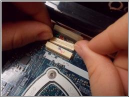
Disconnect all wires connecting the screen to the inside of the computer.
