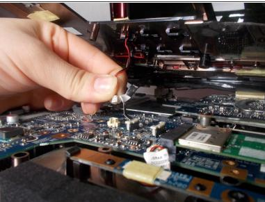
Disconnect all wires connecting the top piece to the bottom.
