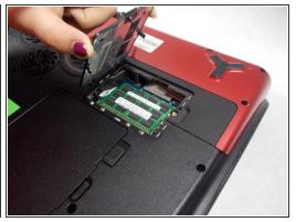
Use a Phillips #0 screwdriver to unscrew the single 8 mm screw and remove the RAM cover.
