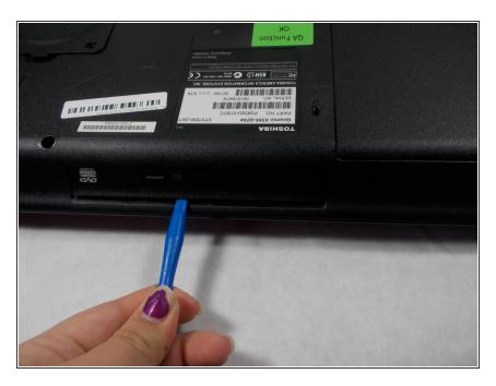
Insert an iFixit opening tool in between the drive and computer body on the bottom edge of the optical drive and pry it out towards you.
