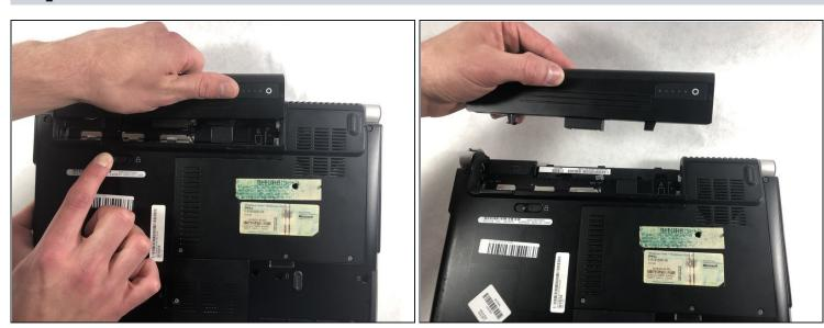
• Lift the computer up and slowly pull the battery straight out from the device.
