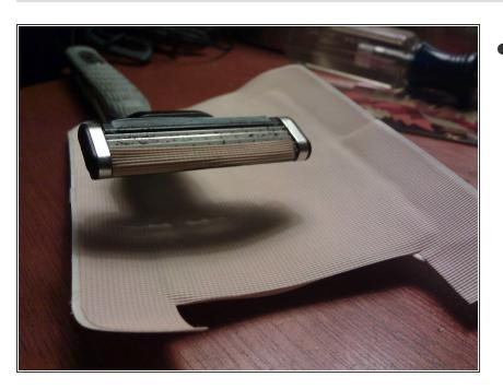
disintegrated) strip from the blade using a knife. Get a waterproof bandaid and cut 4 or 5 thin strips from the sticky part and layer them to make a new strip. Use the smooth-type bandage; not flexible fabric. Then sharpen by stropping on blue jeans. Voila! Shaves just like new. Blow dry after shaving to prevent rust.
