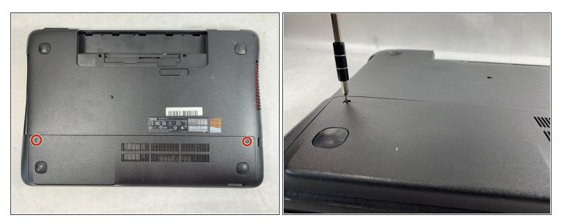
Using a Phillips #000 screwdriver, remove the two 11mm screws that hold the access panel in place.
