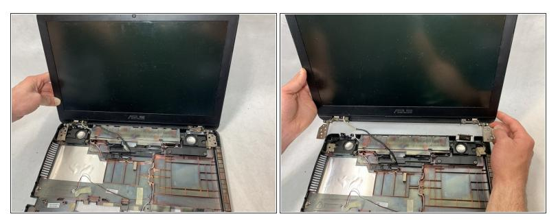
• Lift the display assembly up, separating it from the base of the device.
