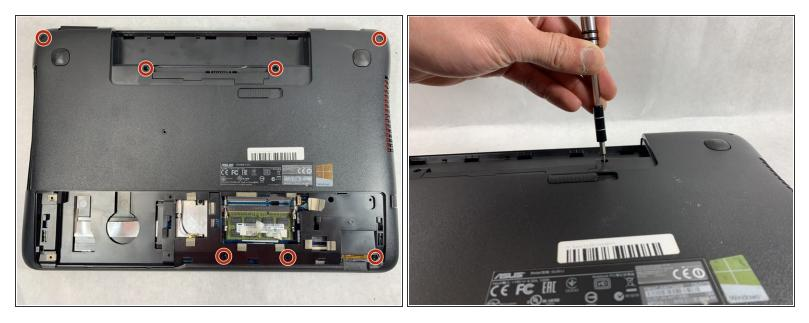
Using a Phillips #000 screwdriver, remove the seven 11mm screws holding lower case to the laptop.
