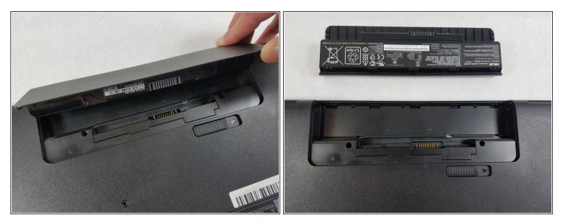
• Grab the battery and remove it from the device.
