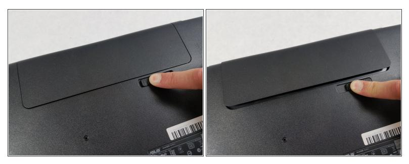
• Move the battery eject button to the right. The battery will be ejected.
