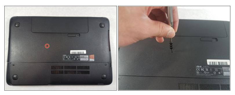
Use a Phillips #000 screwdriver to remove the single 10mm optical drive screw.
