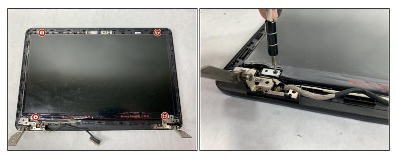
• Remove the four screws using a Phillips #0 screwdriver.
