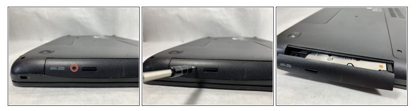
• Insert a probe or paperclip gently into the eject pin hole to eject the optical drive tray.
