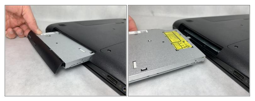
• Gently grasp the optical drive assembly and slide it out of the laptop body.
