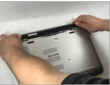
Grab the battery, rotating upwards and away from you. This will remove the battery.
