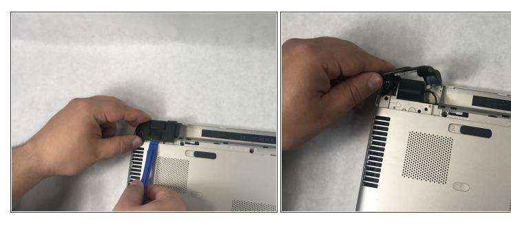
Lift the corner covers off of the computer using a prying tool.
