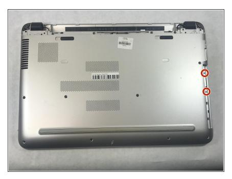
Use the Phillips #0 screwdriver to remove the two 2mm screws.
