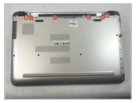
Remove the six 6.5mm screws using a Phillips #1 screwdriver that are located near the top of the laptop.
