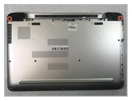
Using the Phillips #1 screwdriver, remove the two 12mm screws located on the hinge covers.
