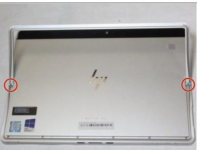
Lift the prop stand approximately 140 degrees from its home position to expose two T5 Torx head screws.
