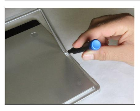
Use the T5 Torx bit to remove both screws from the prop stand pivot points.
