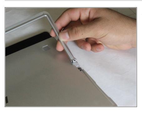
Gently pull the stand away from the device until you can lift the prop stand away from the device.
