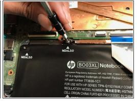
Remove the seven M2xL3.0 screws from around the battery using a Phillips #00 screwdriver.
