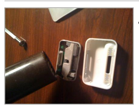
Heat up the adhesive that covers the three screws, so you can unscrew the screws that hold the weight in the base of the dock.
