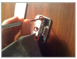
Remove the three screws holding the weight to the bottom plate.
