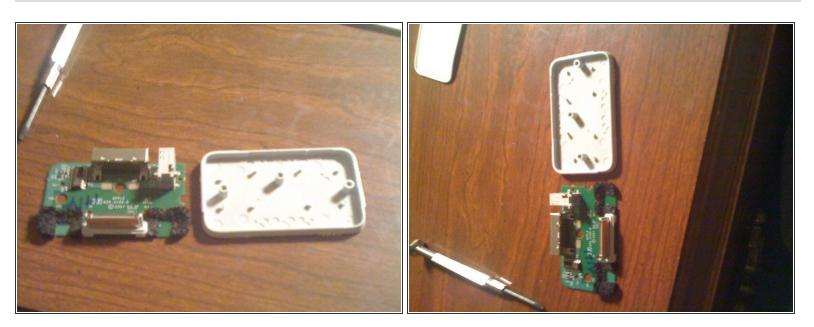
Once done separating the logic board from the bottom plate, you should have 2 parts.
