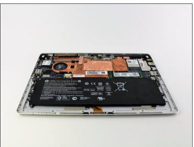
Remove the screen by gently lifting it off of the device.
