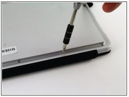
Remove the six 3mm Torx T5 screws underneath the kickstand.
