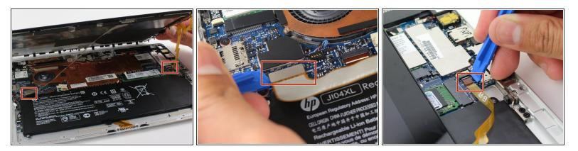
Remove the two connectors on the back of the screen by lifting the connector tabs on the motherboard with a plastic opening tool and pulling gently.
