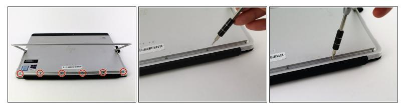
• Remove the six 3mm Torx T5 screws underneath the kickstand.
