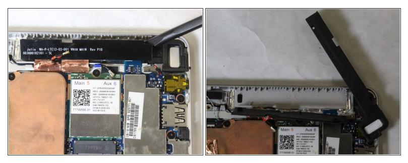
On the right speaker, the black antena piece must be removed before the speaker can be accessed.
