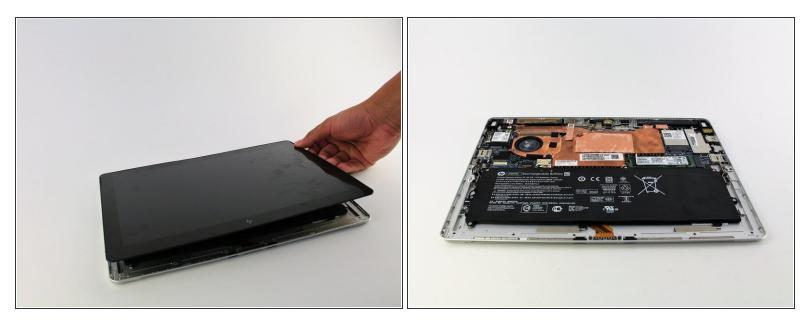
• Remove the screen by gently lifting it off of the device.
