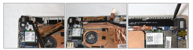
• Use the spudger tool to remove the speakers from the housing.
