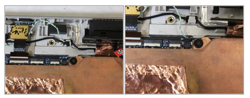
Now remove the green and white wires from the cable management track and the speakers will be completely removed from the device.
