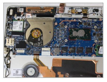
Lift the heatsink off the motherboard.
