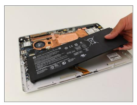
• Lift the battery out of the device.
