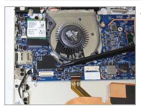
Use a spudger to lift the connection for the fan and disconnect the plug from the motherboard.
