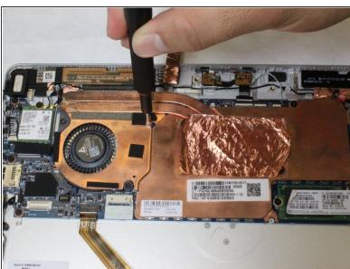
Use Phillips #00 screwdriver to remove seven 3 mm screws.
