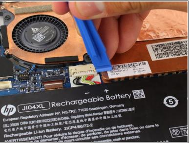
Remove the battery's connector by pushing both sides of the tab towards yourself with a plastic opening tool.
