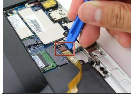
Remove the two connectors on the back of the screen by lifting the connector tabs on the motherboard with a plastic opening tool and pulling gently.
