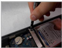
Remove two 4mm Phillips #00 screws that are holding the hard drive in place.
