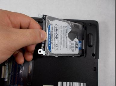
Push the hard drive to the right and push it upward to remove. You may need a spudger or plastic opening tool to assist you with this step.
