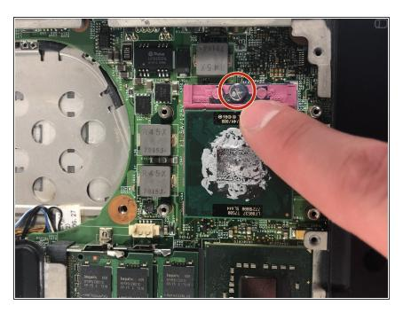
Using the flathead screwdriver, turn the one screw counterclockwise to loosen the CPU, but do not remove the screw.
