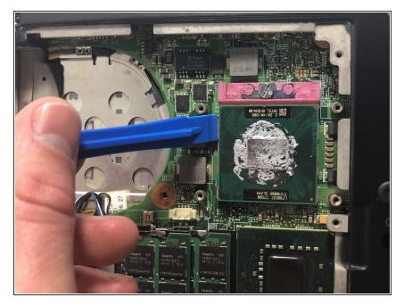
• Using the iFixit opening tool, prop up the CPU.
