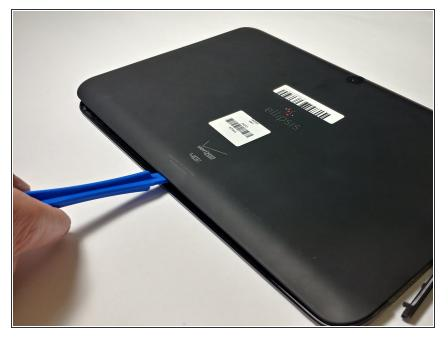
• Follow along the edge of the device to undo all of the retaining clips.
