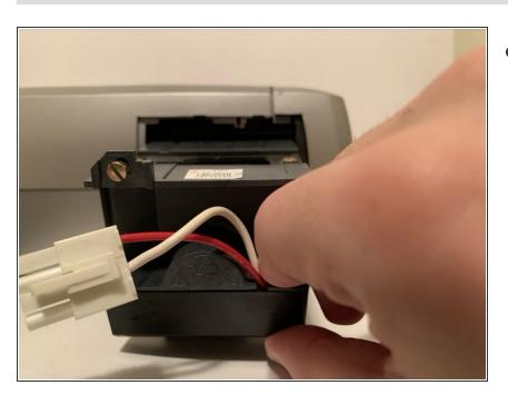
Pull on the bottom plastic tab and remove the lamp by hand.
