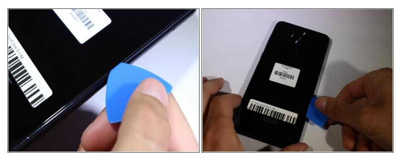
• Use a thin plastic tool to peel the back cover of the phone off. Once the plastic tool has begun to pry the back off, slide the plastic tool around the edges of the phone to separate the adhesive holding the back on. Once all edges of the phone are disconnected, lift the back cover off.
