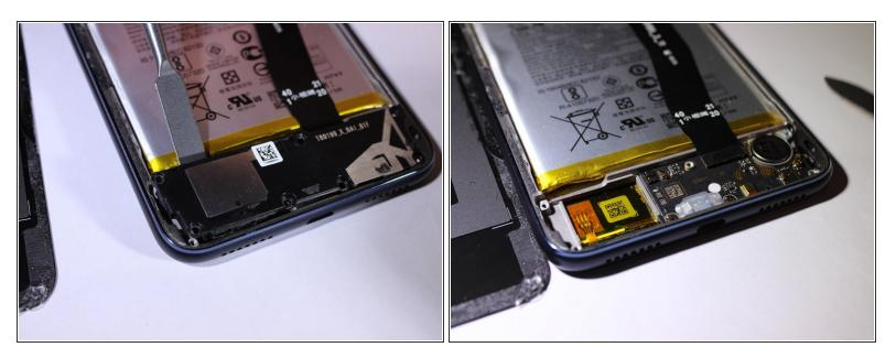
• Use the nylon spudger to pry off the lower cover. Use the opening tool to help lift it off.
