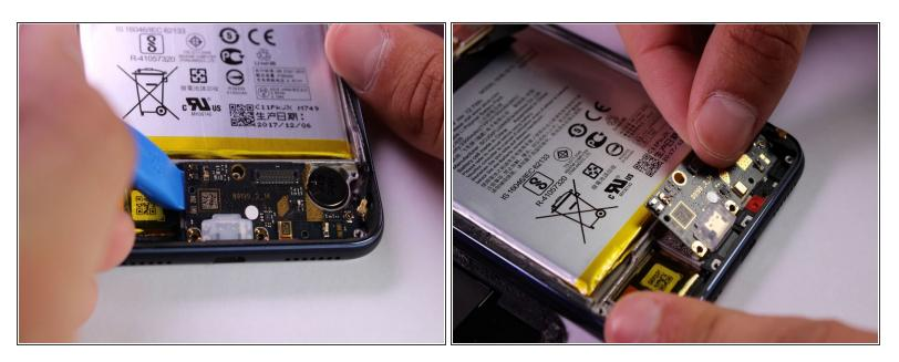
Insert a plastic prying tool on the left side of the charging port. Gently lift up the charging port and then remove using your hand.
