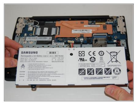
Lift the battery up and out of the case.
