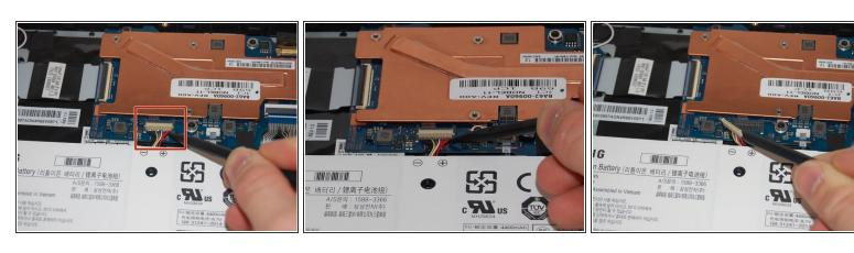
Use the spudger to pry underneath the cable and gently lift the connector up.
