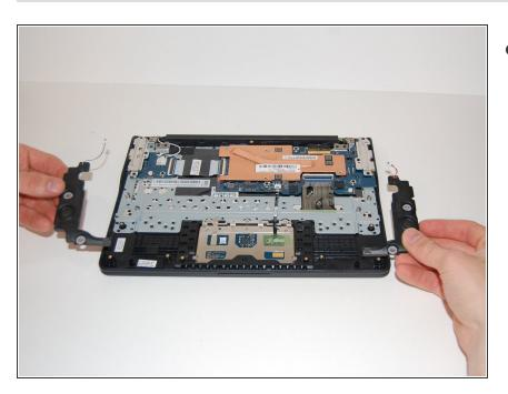
Remove the speakers by lifting them upwards and out of the laptop.
