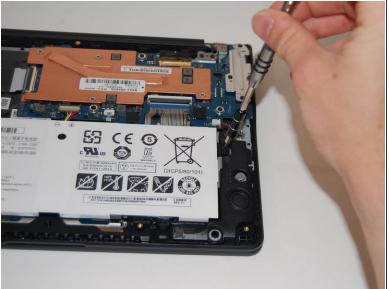
Remove the four 4.6mm screws with the Phillips #00 screwdriver.
