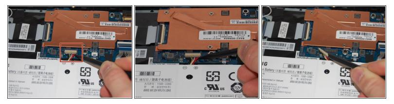
• Use the spudger to pry underneath the cable and gently lift the connector up.
