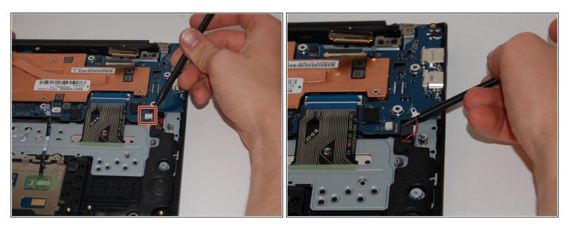
• Remove the right speaker connector using a spudger.
