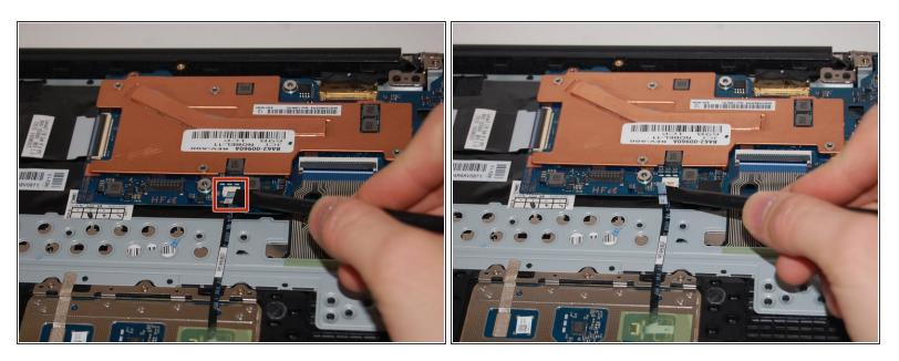
Slide the track pad ribbon cable out from the motherboard using a spudger.
