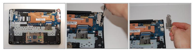
• Remove the three 4.6mm screws from the silver port cover using a Phillips #00 screwdriver.
