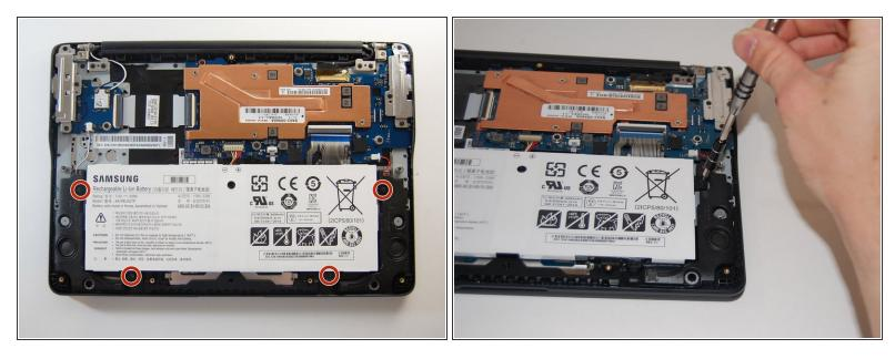
• Remove the four 4.6mm screws with the Phillips #00 screwdriver.
