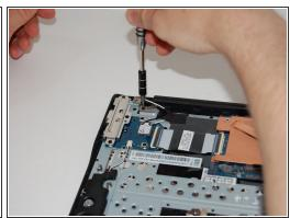
Remove the four 4.6mm screws from the display mounts using a Phillips #00 screwdriver.
