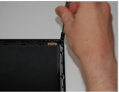
Remove the four 4.6mm screws from the display mounts using a Phillips #00 screwdriver.
