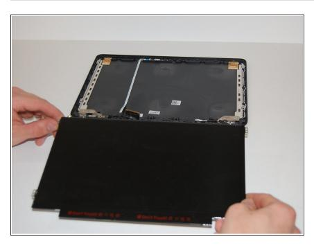
Once the display cable has been removed, lift the screen up and out of the case.
