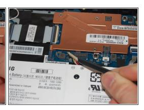
• Use the spudger to pry underneath the cable and gently lift the connector up.
