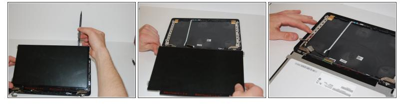
Gently lift the panel up and fold it over to expose the display cable on the backside of the display.
