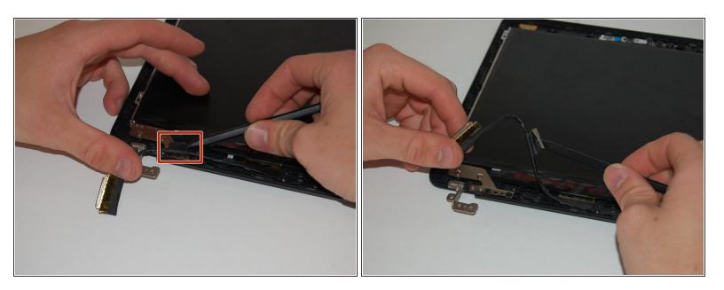
Using the spudger, lift the adhesive tape holding the display cable.
