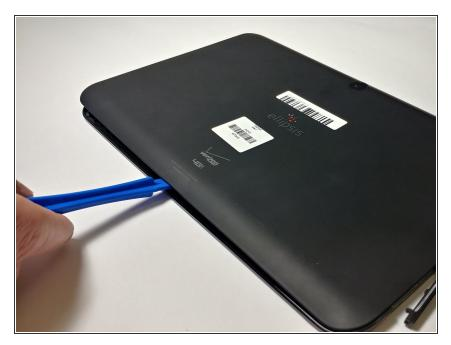
Follow along the edge of the device to undo all of the retaining clips.
