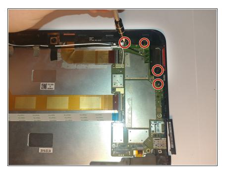
Using a Phillips #00 screwdriver, remove the four M1.5 screws from the right speaker.
