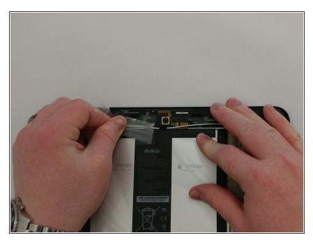
Once you have a hold on the tape, carefully remove it making sure you aren't damaging the battery in the process.
