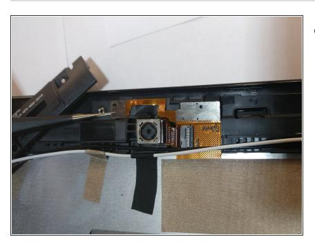
Use a pair of tweezers to lift up the front camera off its locating post.
