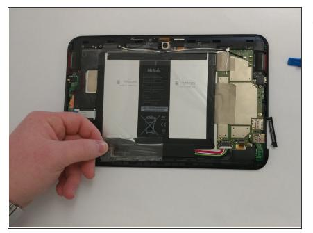
Remove the bottom piece of tape securing the battery making sure you are not peeling up anything else in the process.
