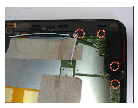
Remove 4 M1.5 screws holding in the labeled LTE module.
