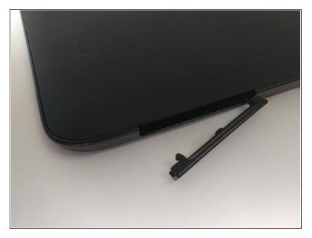
• Open the SD/SIM card cover to start prying off the back cover.
