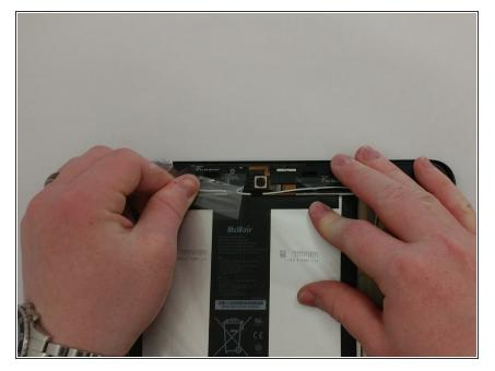
Once you have a hold on the tape, carefully remove it making sure you aren't damaging the battery in the process.
