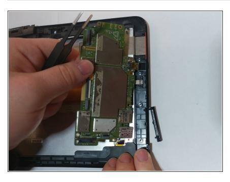
• Once all screws are removed, the motherboard should easily come off the device without any resistance.
