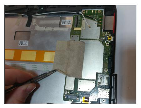
• Remove the non-conductive tape covering two ribbon cables.
