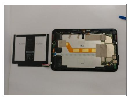
• The battery should be free to come out of the device. Make sure not to bend or damage the battery.
