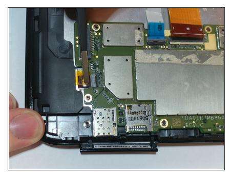
• Unplug the last ribbon cable from the bottom of the motherboard.
