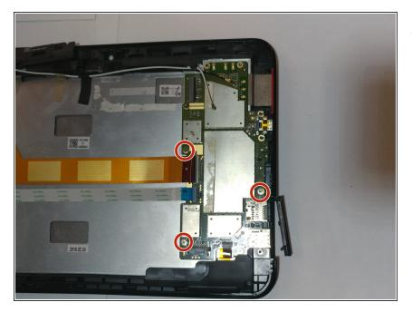
• Remove all M1.5 screws holding in the motherboard.
