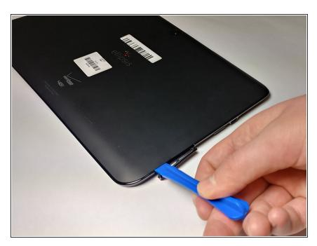
• Start using the iFixit Opening Tool in the SD/SIM area to release the clips holding the back panel on.
