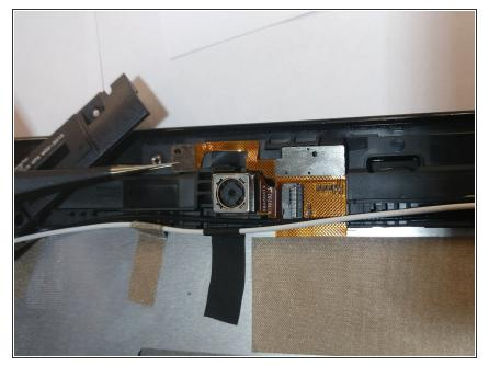
• Use a pair of tweezers to lift up the front camera off its locating post.
