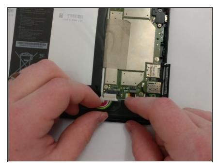
Unplug the battery power connector by sliding the white plastic plug down away from the board.
