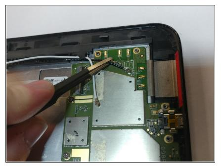
• Use tweezers to pry/disconnect both the black and white antenna cables from the top of the motherboard.
