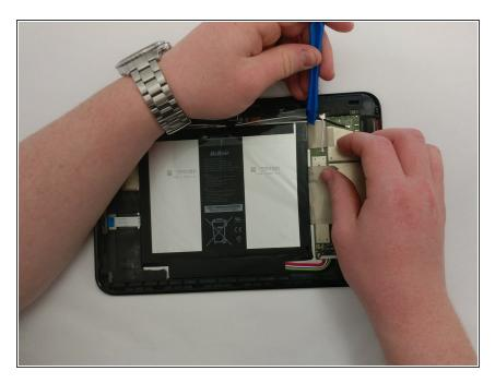
• Remove the top piece of tape using an iFixit opening tool.
