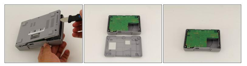
• Remove the back plate from the rest of the console using your hands or the Jimmy tool.
