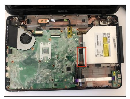
Lift up the flap and there will be two 2 mm Phillips screws beneath that will need to be unscrewed to pull the disk drive out.
