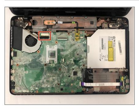
Remove the indicated conduit by gently pulling it away from the motherboard.
