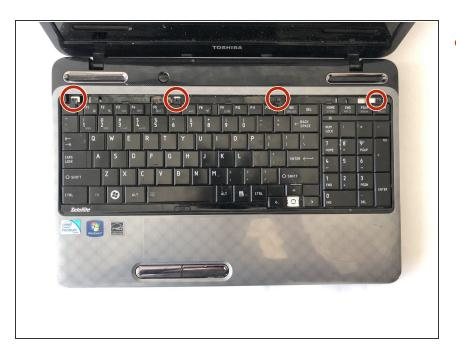
Unscrew the four 4mm Phillips #0 screws beneath the bar.
