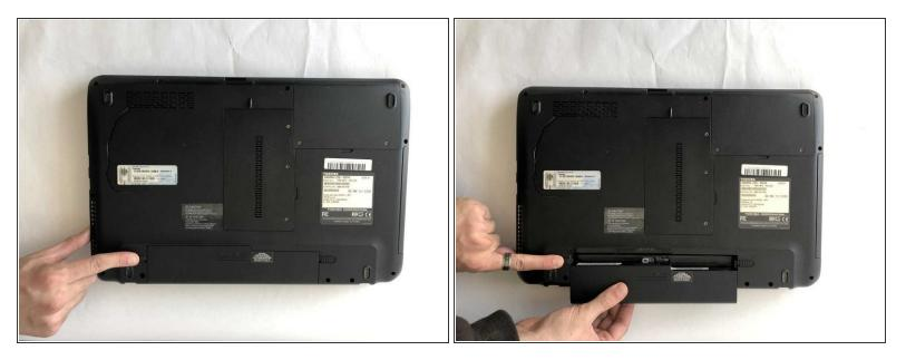
• As a safety precaution, unplug the laptop and remove the battery.
