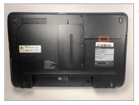
Use the cutaway to lift the panel away from the lap top.
