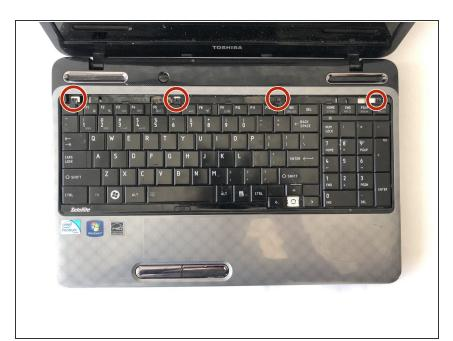
Unscrew the four 4mm Phillips #0 screws beneath the bar.
