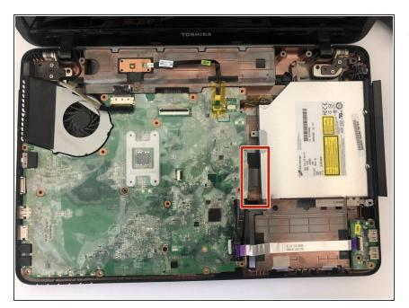
Lift up the flap and there will be two 2 mm Phillips screws beneath that will need to be unscrewed to pull the disk drive out.
