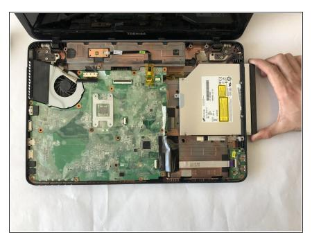
• Now the disk drive will be able to be removed from the motherboard by sliding the drive to the right.
