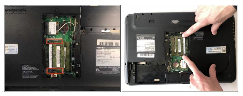
Each RAM stick has two (2) snap locks, one on each end. In the image the bottom snap is obscured by the cable.
