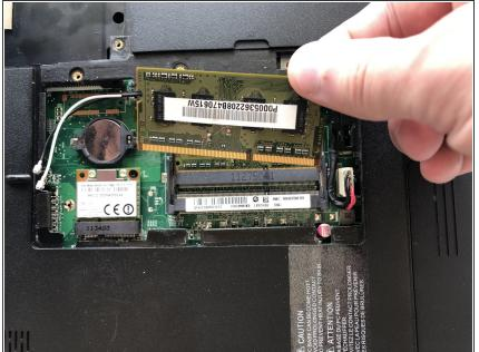
(i) The RAM stick has a notch that is not centered on the stick. Be sure to take note of the RAM stick's orientation for reinstallation
