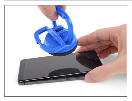
• Carefully open the clamp on the suction cup to release the suction, and remove the suction cup.
