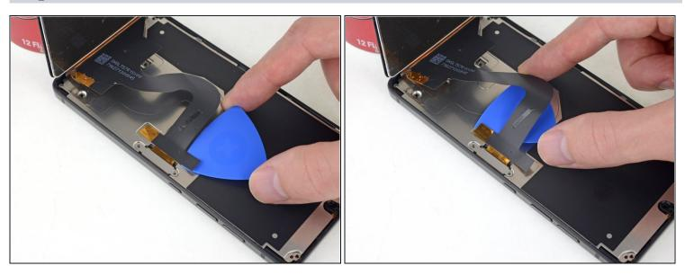
• Carefully slide a pick underneath the display cable to separate the adhesive securing it to the metal shield beneath.
