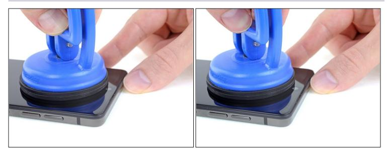
• Pull on the suction cup handle to open a slight gap between the top edge of the display and the Essential Phone's titanium enclosure.
