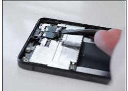
• Use the flat end of a spudger to lift up the clip connectors attached to the rear-facing camera.
