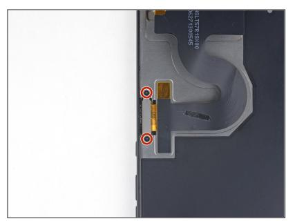
Use a Phillips #00 driver to remove the two 1.5 mm screws securing the display cable.
