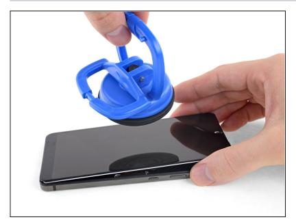
Carefully open the clamp on the suction cup to release the suction, and remove the suction cup.
