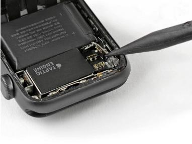
Use the point of a pry tool to disconnect the Force Touch gasket by prying its connector straight up.
