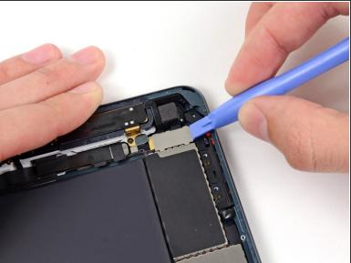
Use a plastic opening tool to push the metal bracket slightly to the left.
