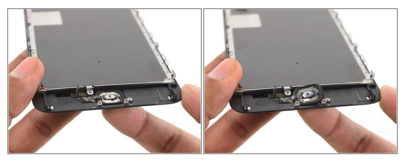
$\bigwedge$  The rubber gasket surrounding the home button is very thin and tears easily.
