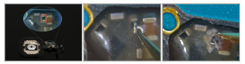
• Find the resistor tied to the home button and remove the protective layer around that resistor.
