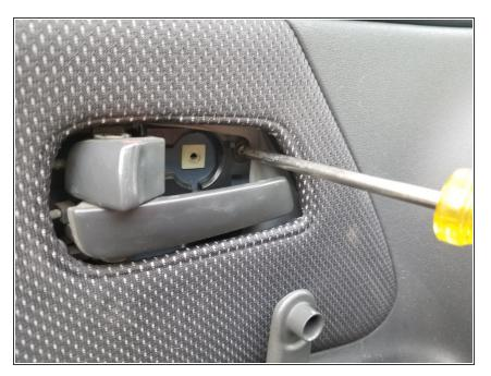
• Remove the screw holding the door handle to the door frame.
