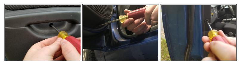
• Remove all screws holding the door panel in place.
