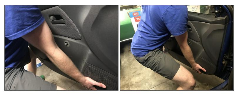
• Remove the door panel by pushing upwards.
