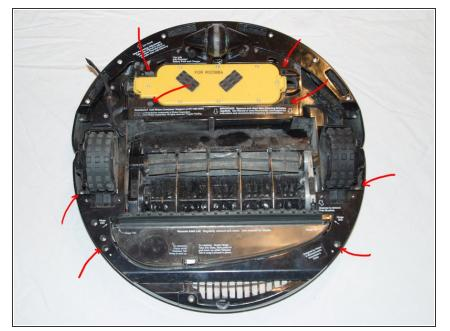
Now go ahead and remove all eight screws. (please excuse the battery in the picture, you should have removed it back in step 1.)
