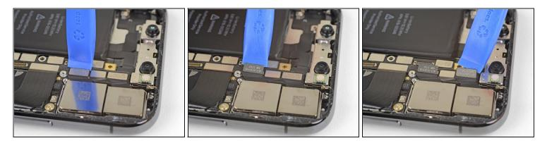
• Use an opening tool or fingernail to disconnect the two camera connectors by prying them straight up from their sockets.
