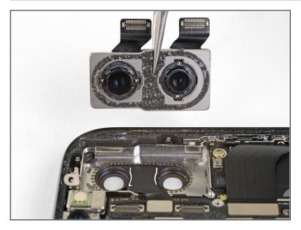
Remove the rear-facing camera module.
