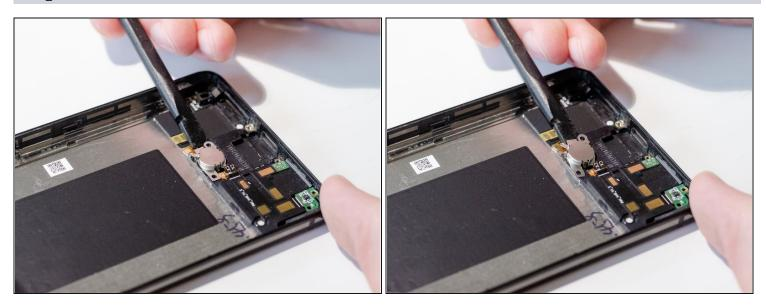
• Using the flat edge of a spudger, lift off the vibrator cap from the device.
