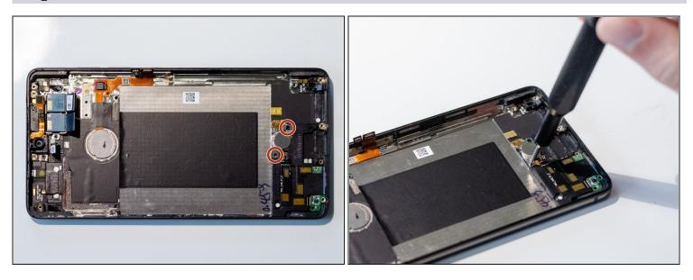
• Remove the two 1.25mm screws that hold on the vibrator cap using a Phillips #000 screwdriver.
