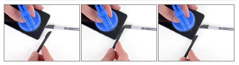
• Insert a halberd spudger no more than 1 mm under the display, and cut the adhesive all along the top edge.
