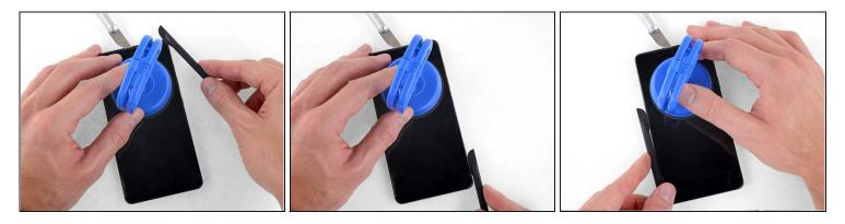
• Continue carefully separating the adhesive at the top corners and down both sides of the display.
