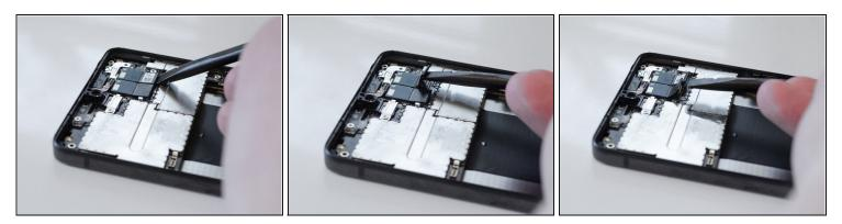
• Use the flat end of a spudger to lift up the clip connectors attached to the rear-facing camera.
