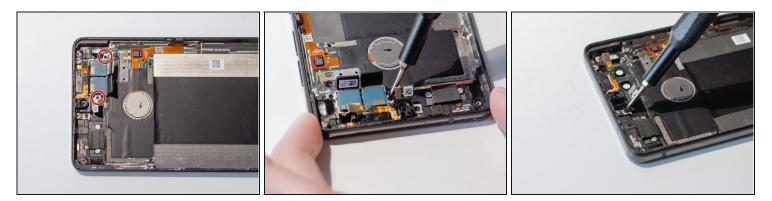
• Unscrew the two 1.65mm screws holding the camera components using a Phillips #000 screwdriver.
