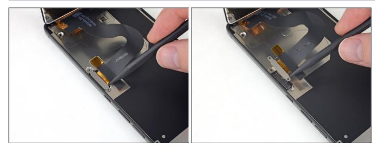
• Use the point of a spudger to pry the display cable <u>pop connector</u> straight up from its socket.
