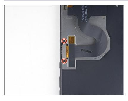
• Use a Phillips #00 driver to remove the two 1.5 mm screws securing the display cable.
