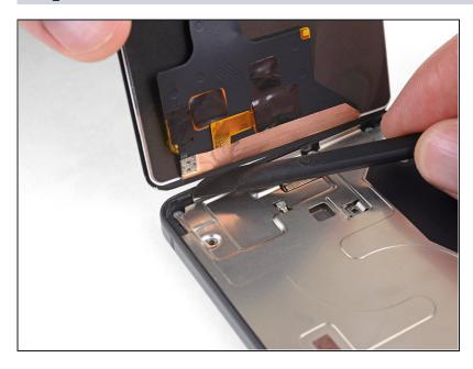
• Use your halberd spudger to carefully separate any remaining adhesive along the bottom edge of the phone.
