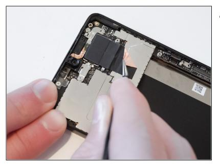
• Use a tweezer to remove the tape covering the rear cameras from the motherboard.
