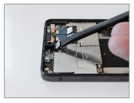
• Use the flat end of a spudger to lift up the clip connectors located near the front-facing camera.
