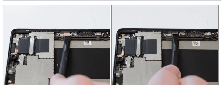
• Use the flat end of a spudger to lift up the tab of the connector from the motherboard.
