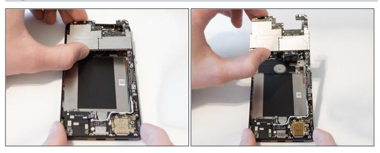
• Carefully lift the motherboard out of the phone. This may require some fidgeting to unhook the motherboard.
