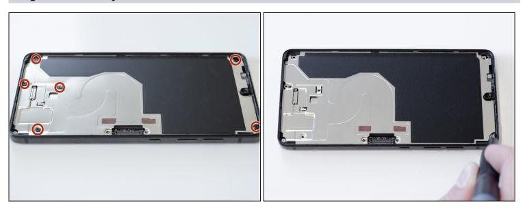
• Use a Phillips #000 driver to remove the six 3.4mm screws holding on the back panel.
