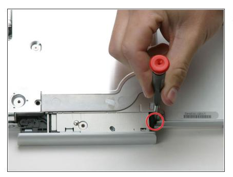
Pull the optical drive out just enough so that you can access and remove a Phillips screw near the battery compartment.
