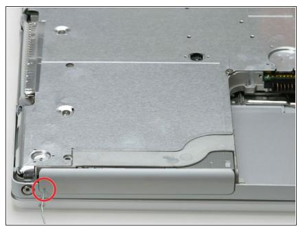
• Use a straightened paperclip to open the optical drive tray.
