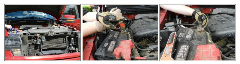
• Use an adjustable wrench to disconnect the negative power from the battery (Turn counterclockwise then lift).
