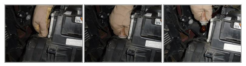
• Remove the headlight bulb (Turn counterclockwise then lift).
