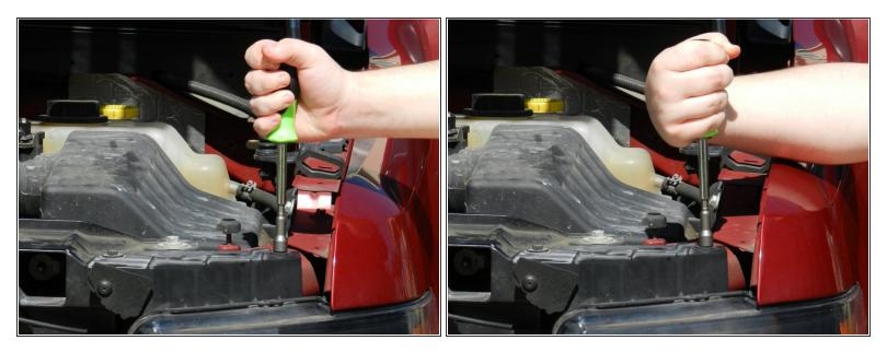
Use the socket wrench with the 10 mm socket to unscrew each socket (Turn counterclockwise).
